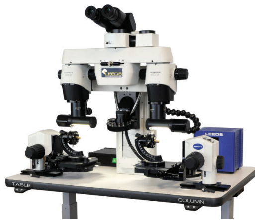
Figure 4. Comparison microscope from Leeds Forensic Systems. (Reproduced with permission of Leeds Forensic Systems: Minneapolis, MN.)
